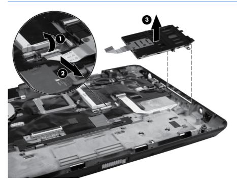
4. Remove the Bluetooth cable by disconnecting the ZIF cable (1) securing the Bluetooth module to the system board and thn lift the cable (2).
